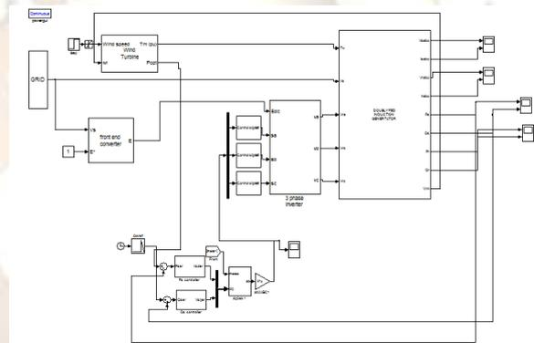
Fig.2: DFIG with PI CONTROLLER
