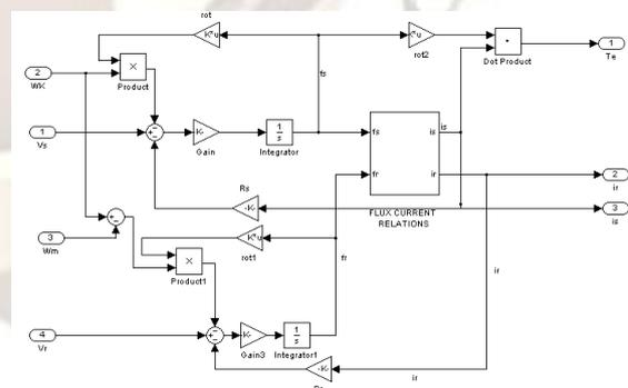
Fig.3: Dynamic Model of Induction Machine in Arbitrary Reference Frame
