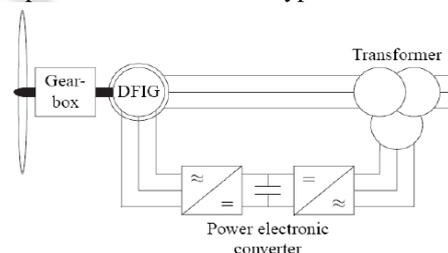
Fig 1. Wind turbine with a doubly-fed induction generator (DFIG)
