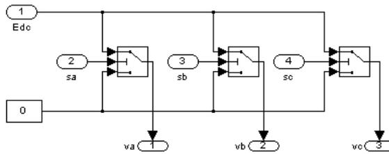
Fig.4: Simulink Diagram for Rotor Side Converter
