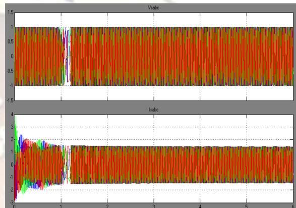
Fig.8: Stator Output Voltage and Current using PI controller
