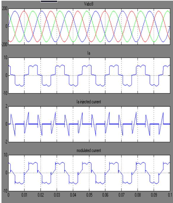
Fig 10 output waveforms with current injection for phase ‘a’
