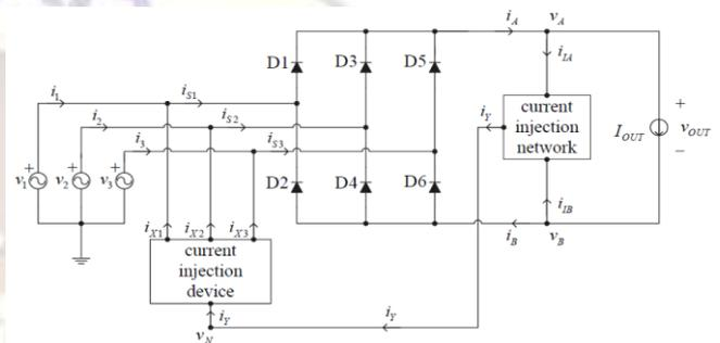
Fig.1 Proposed rectifier block diagram
