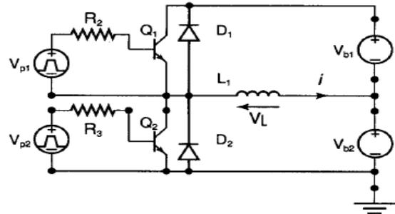
Figure 3 Half bridge inverter
