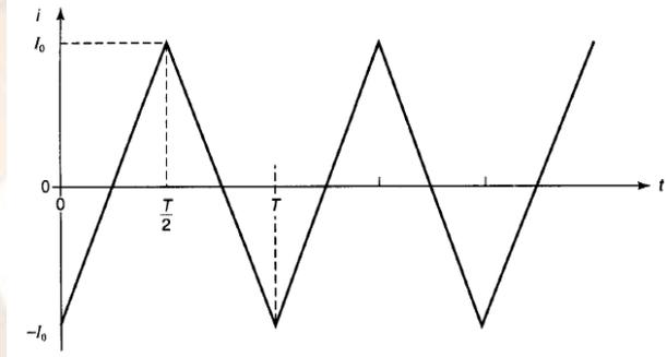
Fig 4 waveform of the half bridge inverter
