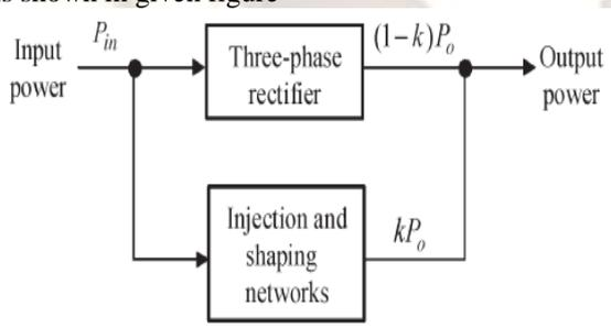
Fig. 11 power flow diagram of converter.
