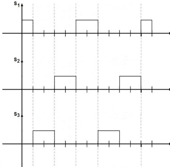
Fig.6. control signals for the switches in the current injection device
