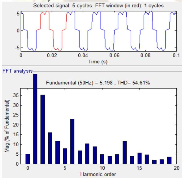
Fig 14. FFT analysis before current injection
