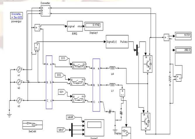
Fig. 9 Simulink diagram for proposed converter
