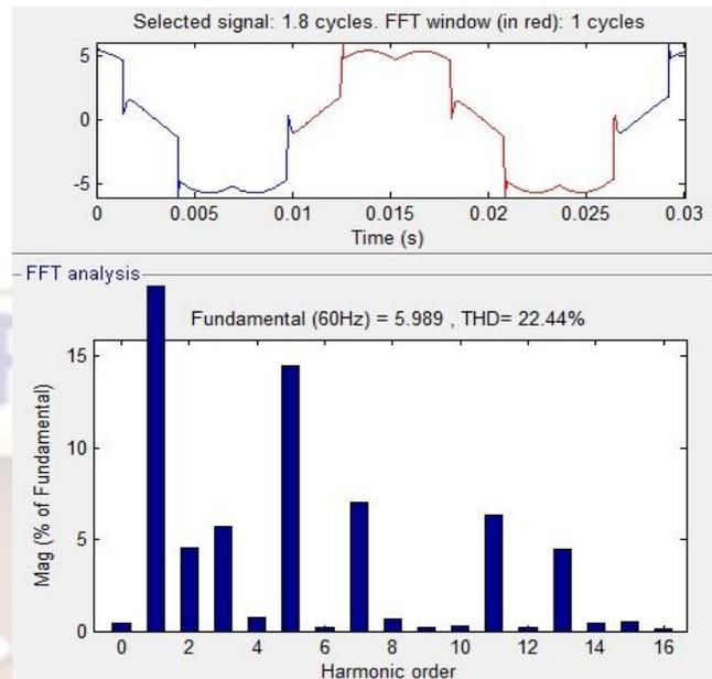
Fig15. . FFT analysis after current injection
