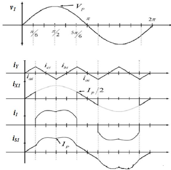
Fig 2: Waveforms of the proposed converter
