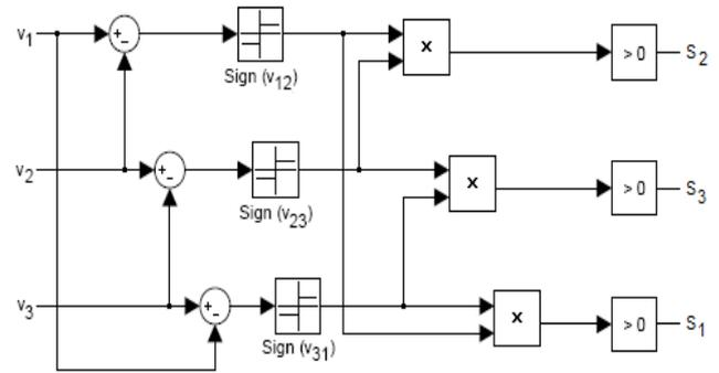
Fig. 7 control signals for injection device
