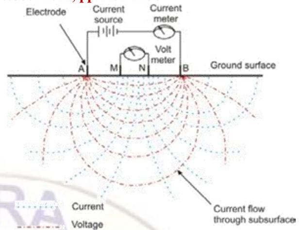
Fig.5: The basic principles of Schlumberger device
