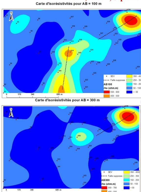
Fig. 7: Kriged contour maps of the apparent resistivity for various Schlumberger electrodes spacing
