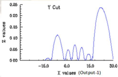
Fig.2(a) multi beam splitter of hexagonal structure of linear SF57 (X-Z plane)
