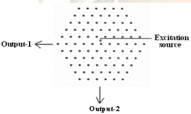
Figure 1. Hexagonal structure of PCFs
