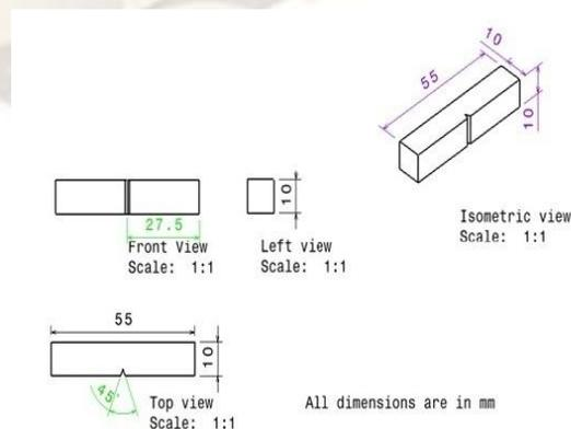
Fig. 3 Charpy Impact Test Specimen
