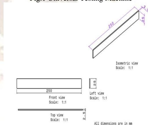
Fig. 2 Tensile strength test specimen
