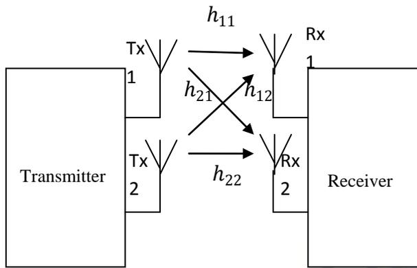
Figure:1. 2 x 2 MIMO system model
