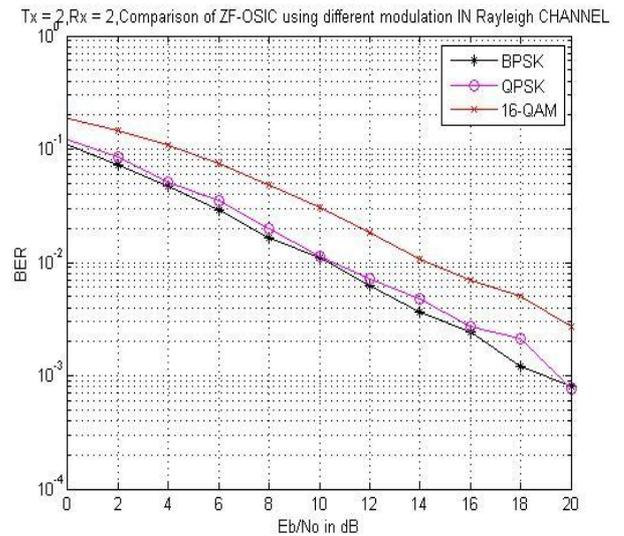
Figure.5 Comparison of ZF-OSIC using BPSK
