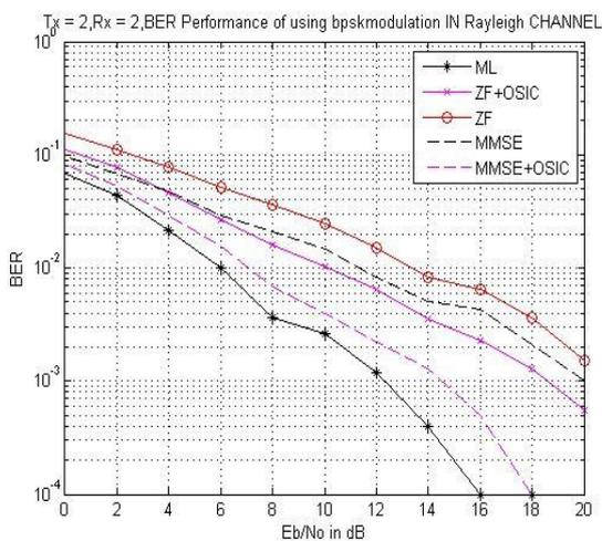
Fig.9 Comparison using different detection technique using BPSK modulation
