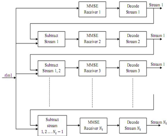
Figure.3 SIC MMSE Detector
