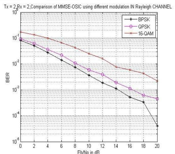
Figure.7 Comparison of MMSE-OSIC using BPSK
