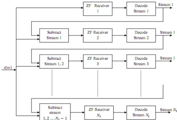
Figure.2 SIC Zero Forcing Detector
