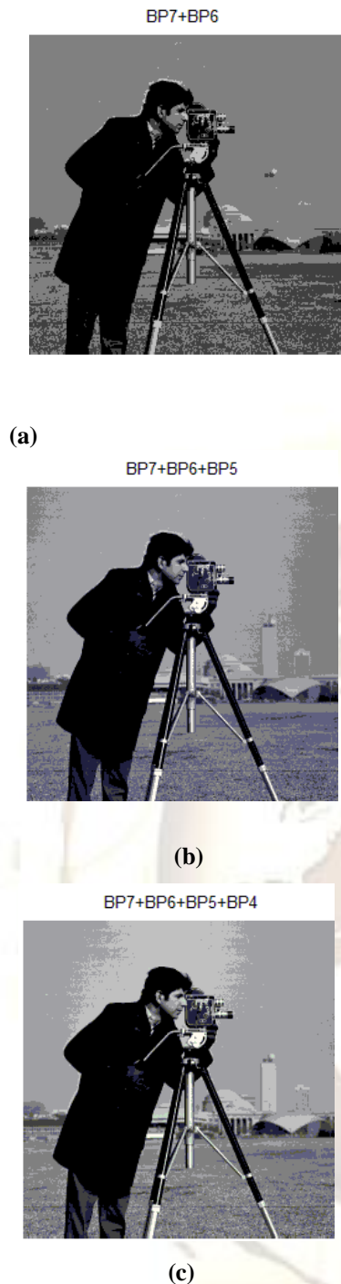
Fig. 2: The effect of various Slice Combinations BP7 – Most Significant Bit plane BP0 - Least Significant Bit plane (a) Image representing Bit plane 7 +Bit plane 6 (b) Image representing Bit plane 7 + Bitplane 6 + Bitplane5 (c) Image representing Bit plane 7+Bit plane 6+Bit plane 5+Bitplane 4
