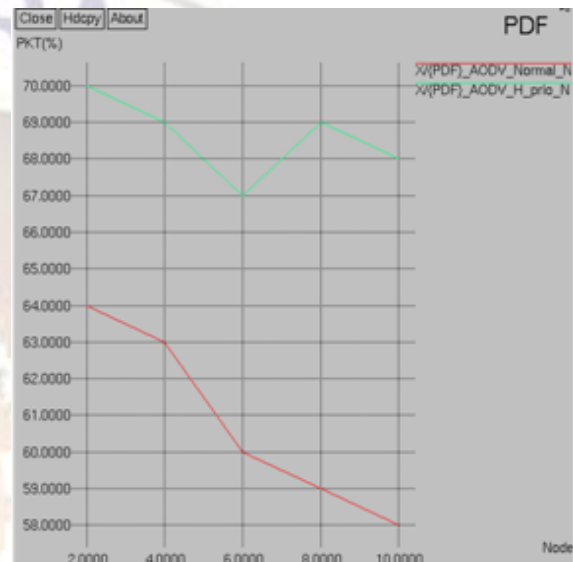
Graph 4: data packet delivery ratio versus number of nodes for priority and priority-less vehicles.
