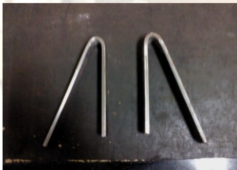
Figure 11: Bend test specimen ( GTAW)
