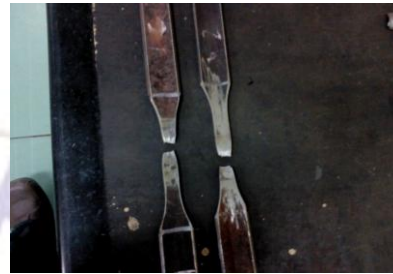
Figure 10: Tensile test specimen (GMAW)
