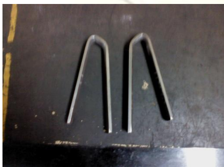
Figure 12: Bend test specimen ( GMAW)
