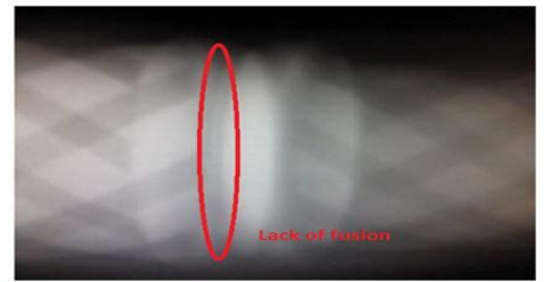
Figure 18: Lack of fusion
