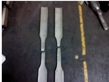
Figure 9: Tensile test specimen (GTAW)
