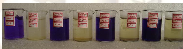
Photo 4: Effect of initial dye concentration on photocatalytic degradation of Violet GL2B [CaO = 0.2 g/100ml, pH = 10].
