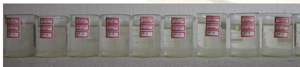
Photo 3: Effect of pH on photocatalytic degradation of Violet GL2B at irradiation time 120 minutes [CaO = 0.2g/100ml, Violet GL2B= 30 mg/L].
