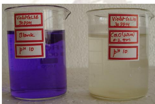
Photo 5: Sunlight irradiation on photocatalytic degradation of Violet GL2B using CaO [(Dye/CaO/sunlight) CaO = 0.2 g/100ml, Violet GL2B=30mg/L, pH = 10].
