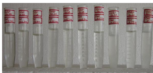
Fig 6: Effect of concentration of CaO on photocatalytic degradation of Violet GL2B at 120 minutes [Violet GL2B=30mg/L, pH=7].
