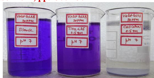
Photo 1: Effect of photocatalytic degradation of Violet GL2B at 120 minutes. [Violet GL2B=30mg/L, pH=7, TiO_2 =0.5 g, CaO=0.5 g].
