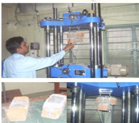
Figure 6 – Testing of brick joint pull strengths
