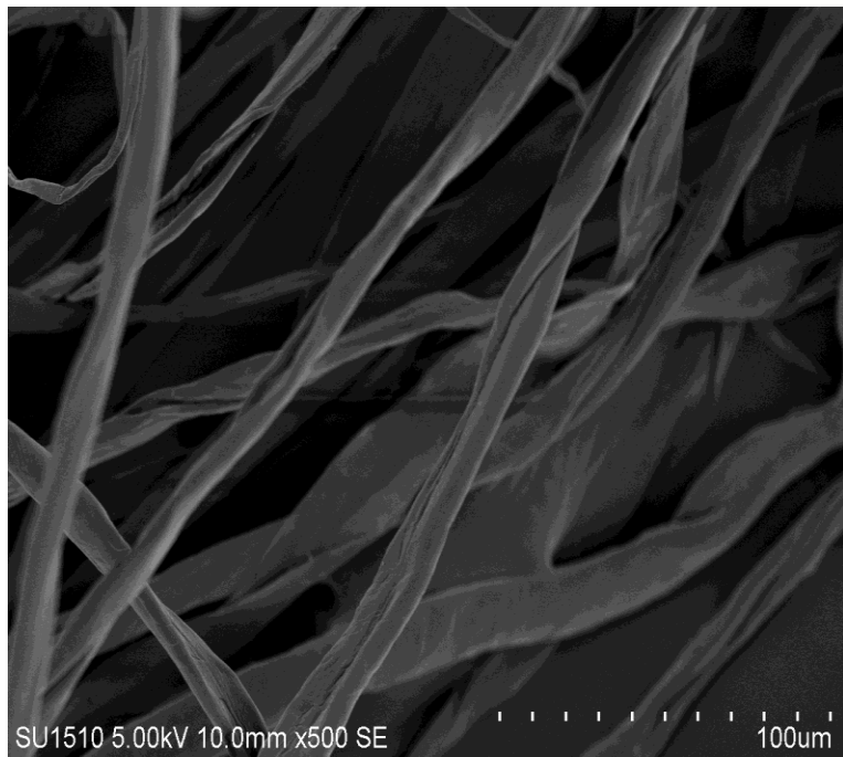
Figure 1: SEM of RCF-Raw Cotton fiber
