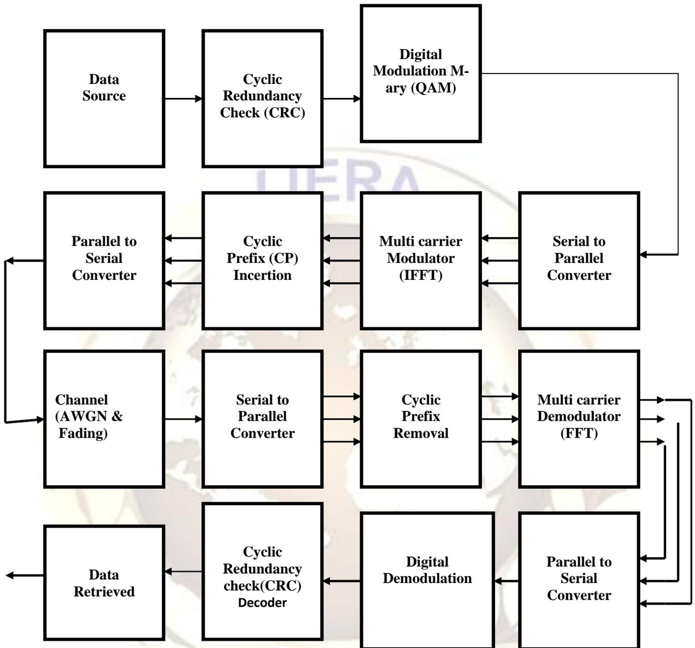
Figure-a: A block diagram of Cyclic Redundancy Check (CRC) encoded WiMAX communication system
