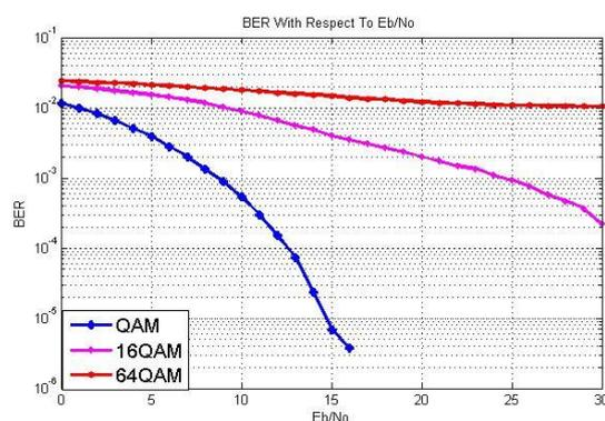
Figure-d: BER simulation of an Cyclic Redundancy Check (CRC) encoded in QAM,16-QAM and 64-QAM modulation schemes in an Rayleigh channel
