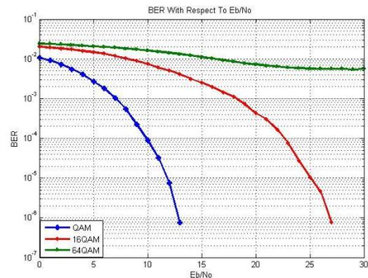
Figure-e: BER simulation of an Cyclic Redundancy Check (CRC) encoded in QAM,16-QAM and 64-QAM modulation schemes in an Rician channel.
