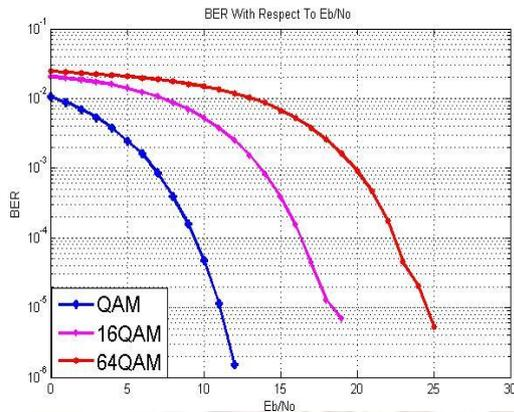
Figure-c: BER simulation of an Cyclic Redundancy Check (CRC) encoded in QAM,16-QAM and 64-QAM modulation schemes in an AWGN channel
