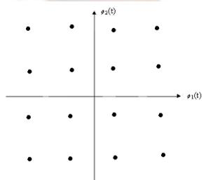
Figure-b: Constellation diagram of an M-ary QAM (M=16) signal set [8].
