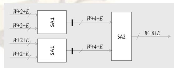
Fig. 8. Pipelined shift-adder tree. E = \log_2 N
