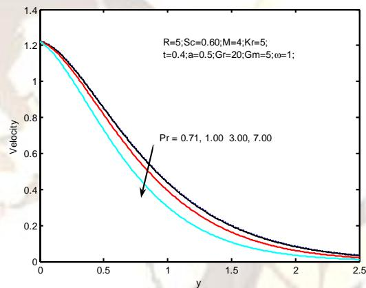
Fig.7. Effects of Prandtl number on velocity profiles.
