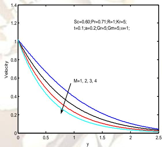
Fig. 1. Effects of magnetic parameter on velocity profiles.
