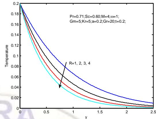
Fig.12. Effects of radiation parameter on temperature profiles.
