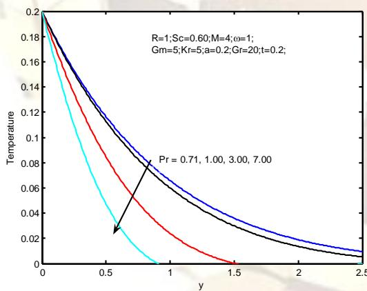
Fig.11. Effects of Prandtl number on temperature profiles.
