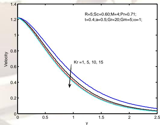
Fig.8. Effects of chemical reaction parameter on velocity profiles.
