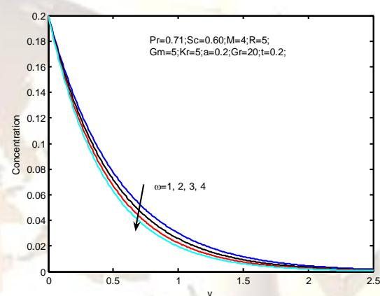
Fig.13. Effects of frequency of excitation on concentration profiles.
