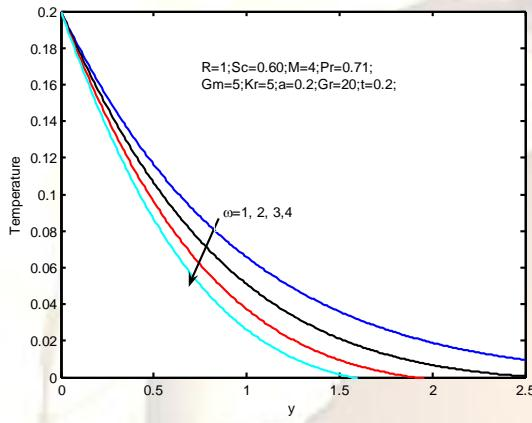
Fig.10. Effects of frequency of excitation on temperature profiles.
