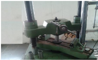
Fig.2 (B) Test cylindrical shell compressed axially on UTM
