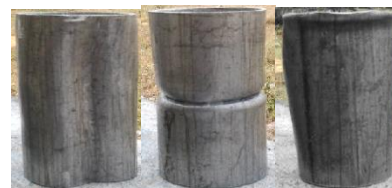
Fig. 6.2.A Deformed shapes--- plain cylindrical shell, with a longitudinal dent and a circumferential dent
