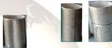
Fig.1 (a). (b) (c) Plain cylindrical shell with longitudinal and circumferential dent
