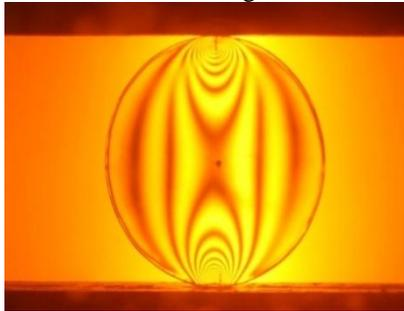
Fig. 14 Isochromatic Fringe pattern for calibration disc
