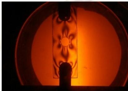
Fig.15. Isochromatic Fringe pattern for circular cutout.
