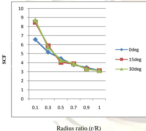
Fig.10. SCF with respect to rotation for triangular cutout
