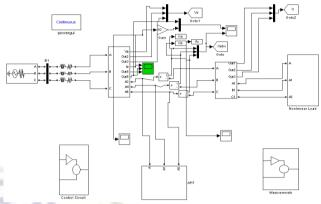
Figure-8 Matlab/Simulink power circuit model of DSTATCOM
