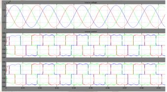
Figure-9 Source voltage, current and load current without DSTATCOM
