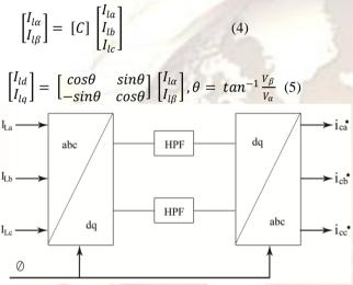
Figure-2 Block diagram of SRF method
