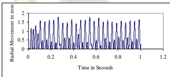
Fig. 6 Cu particle radial movement for 400kV with analytically calculated field
