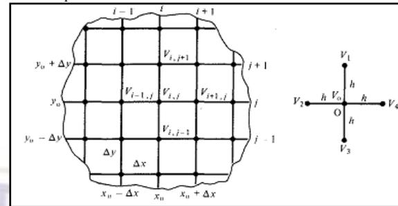
The finite difference approximation to poisson's equation applied to Gas Insulated Busduct solution region for five-node is:
