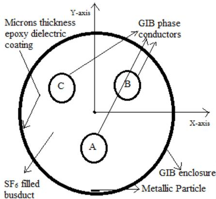
Figure 1. Typical three phase common enclosure Gas Insulated Busduct
