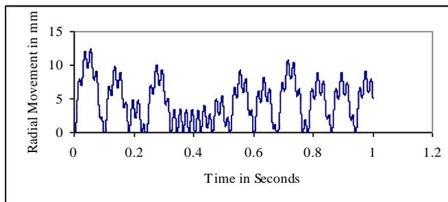
Fig.8 Cu particle radial movement for 400kV with FEM calculated field
