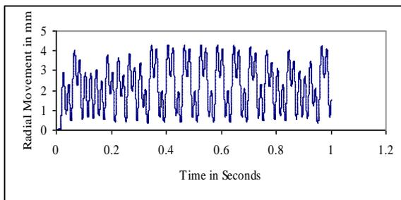
Fig.3 Al particle radial movement for 400kV with analytically calculated field
