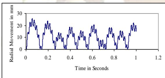
Fig.5 Al particle radial movement for 400kV with FEM calculated field
