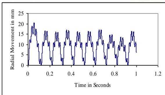
Fig.4 Al particle radial movement for 400kV with FDM calculated field
