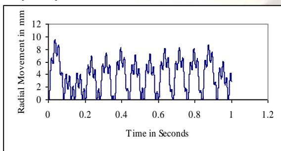
Fig.7 Cu particle radial movement for 400kV with FDM calculated field
