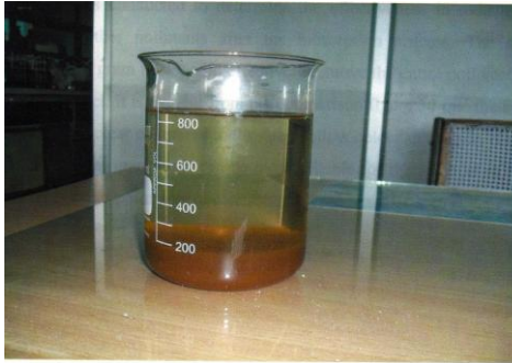
FIGURE.27. SETTLING OF SLUDGE
