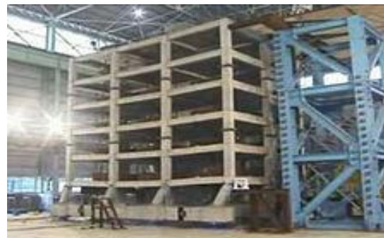
FIGURE.2. SNAPSHOT FROM SHAKE-TABLE VIDEO OF A 6-STORY NON-DUCTILE CONCRETE BUILDING DESTRUCTIVE TESTING
