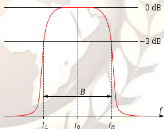
Fig.1 A diagram showing magnitude transfer function versus frequency for a band-pass filter
