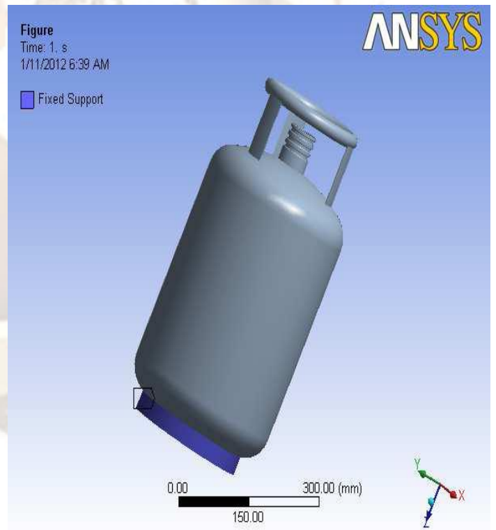
The fixed support is given on the bottom of the cylinder.
