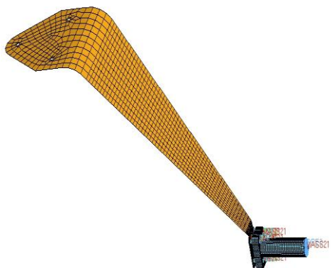
Figure 2.2: 3D-meshed model of landing gear’s leg
