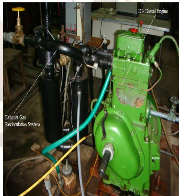
Fig. 1: Shows the experimental set up consisting of DI Diesel Engine with EGR system
