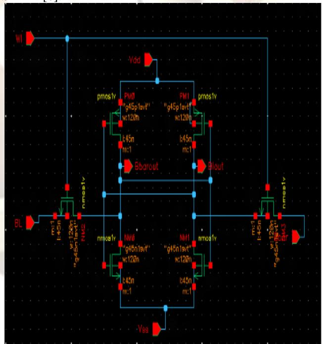
Figure 1: 6T SRAM cell
