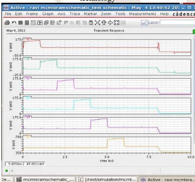
Figure 10: Transient response of (8 X 8) SRAM cell array
