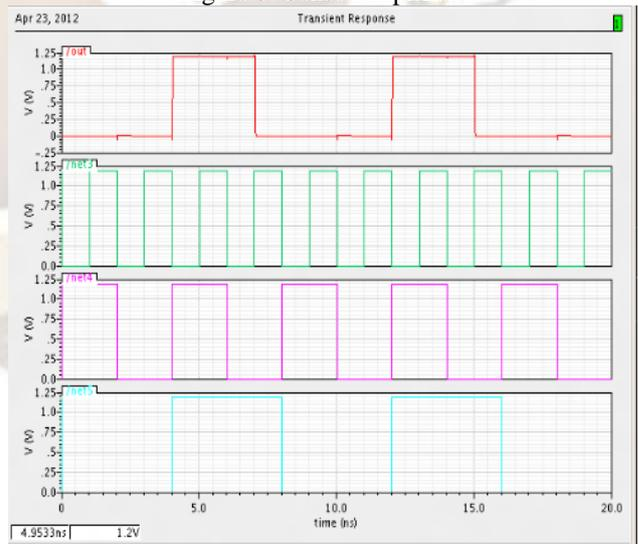
Figure 4: Transient response of Sense Amplifier
