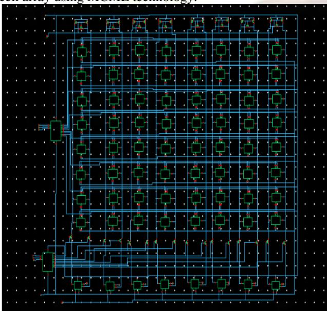
Figure 9: (8 X 8) SRAM cell array using MCML technology
