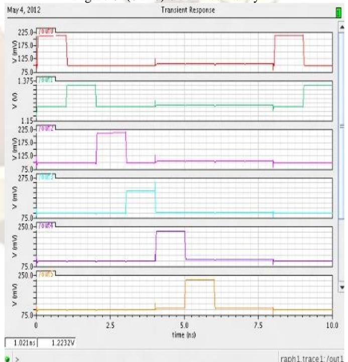
Figure 8: Transient response of 8 X 8 SRAM cell array 3.1 (8 X 8) SRAM ARRAY USING MCML
