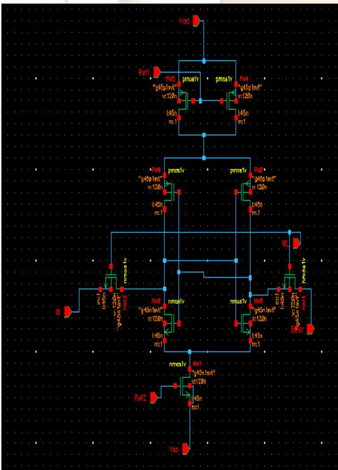
Figure 2: SRAM cell using MCML
