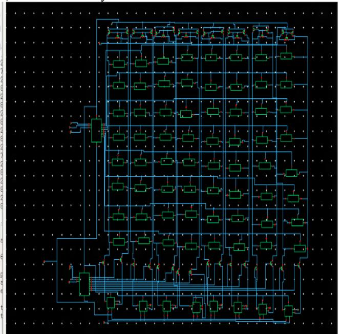
Figure 8: (8 X 8) SRAM cell array
