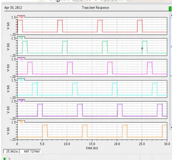
Figure 6: Transient response of 3 to 8 decoder
