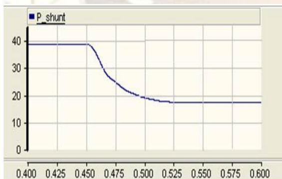
Fig. 22: active power injected by shunt inverter to load
