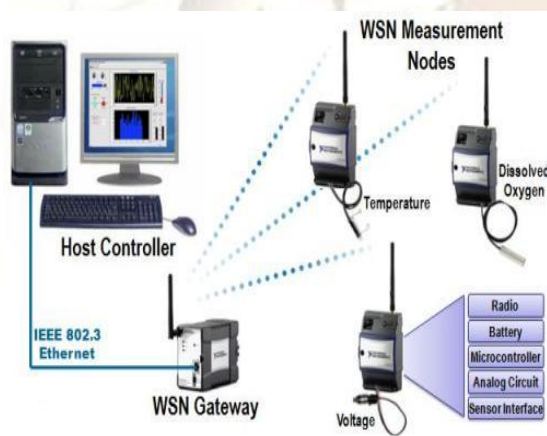
Figure 1: Common Wireless Sensor Network Architecture
