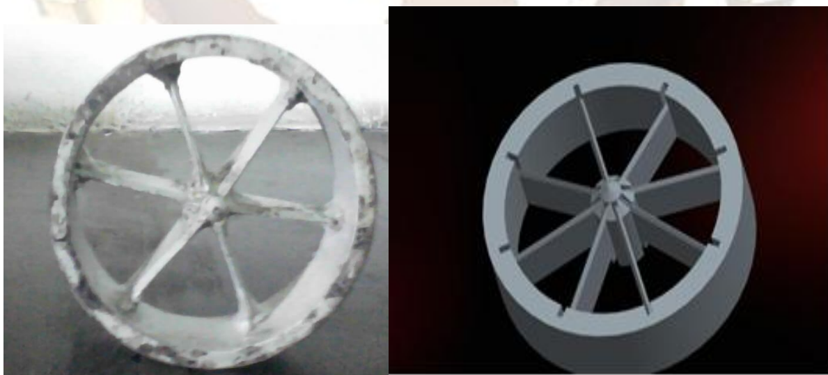
Figure 3:- Actual working Die of splitter, Cad model of splitter.
