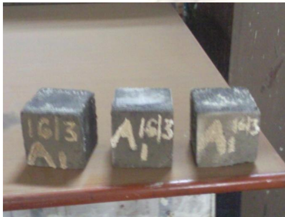
3. first batch of cube specimens casted
