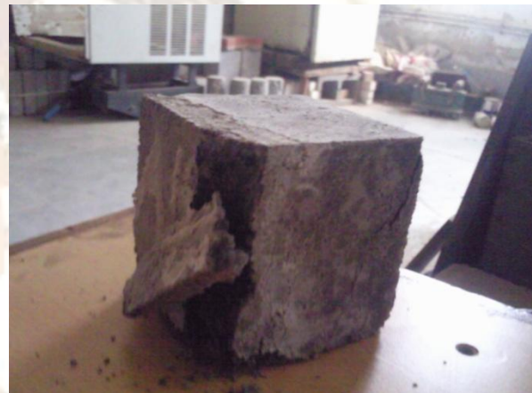
5. specimen after compressive failure
