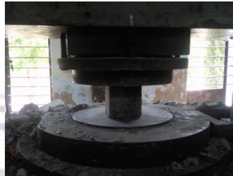
4. specimen tested for compressive strength
