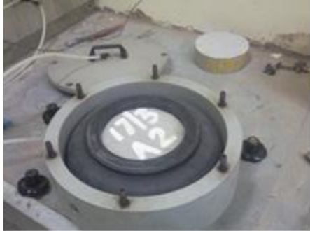
6. cylindrical specimen for permeability testing
