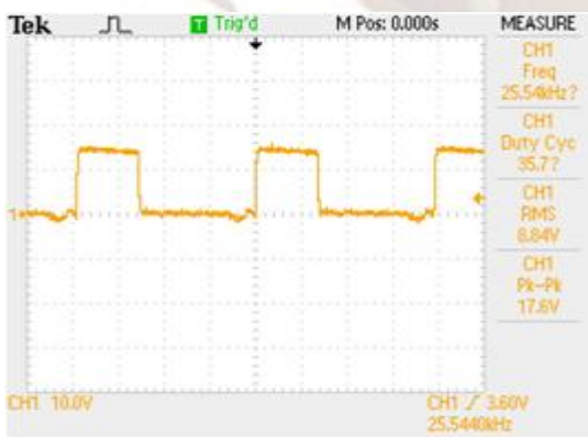
Fig.8. Switching pulse from TLP 250 for lower side switch
