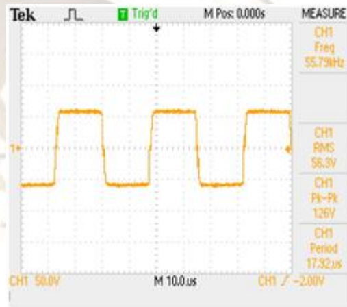
Fig.10. Upper side secondary voltage
