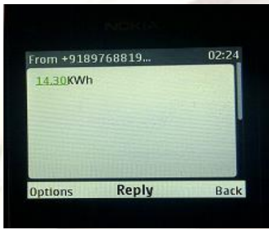
Fig 6.2: SMS received by customer from meter
