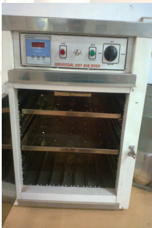
Fig 1 Universal hot air oven
