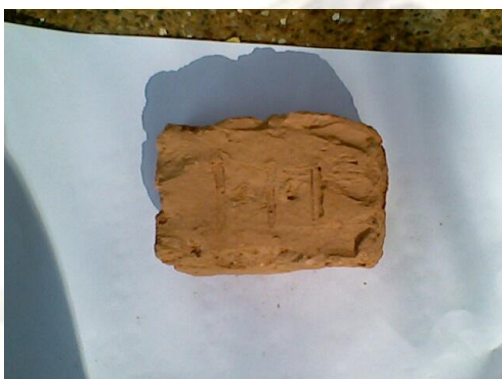
FIGURE.5 BRICK SPECIMEN WITH WTP SLUDGE AND BRICK EARTH
