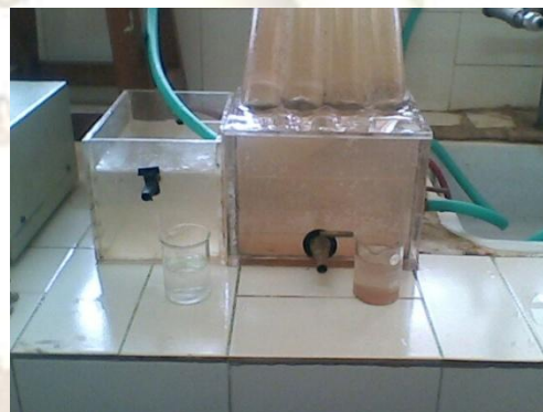
FIGURE.2 TUBE SETTLER UNIT ALONG WITH TREATED WATER COLLECTED IN THE TANK.
