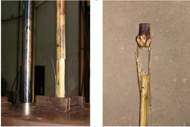
Fig. 6 Smashing and Slip Failure at the Grip (Sample-1)
