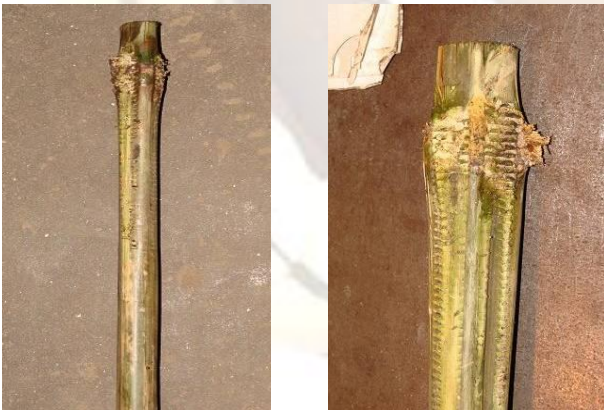
Fig. 8 Slip Failure at the Grip (Sample-3)
