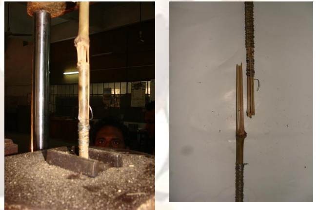
Fig.10 Typical Tensile Failure at Knot between Grips
