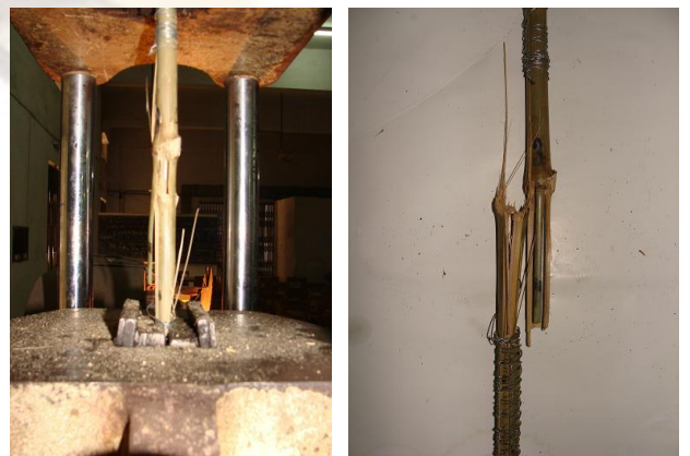
Fig.10 Typical Tensile Failure at Knot between Grips
