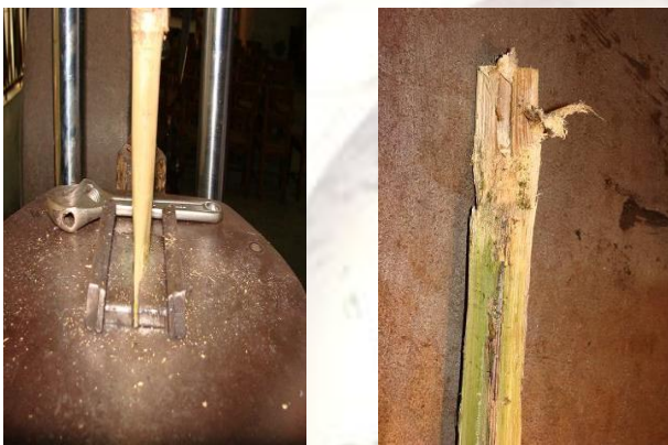
Fig. 7 Smashing and Slip Failure at the Grip (Sample-2)
