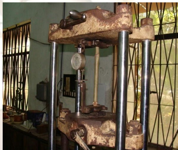
Fig. 5 Use of Compressometer in Tension Test of Finished Bamboo Twig
