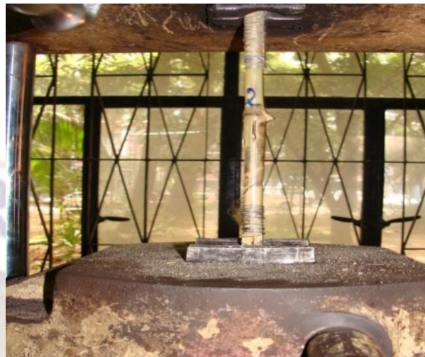
Fig. 4 Bamboo Twig Under Tension Test
