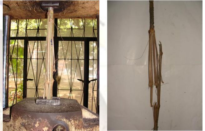
Fig. 9 Typical Tensile Failure at Knot between Grips (Sample-1)
