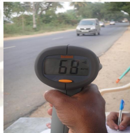
FIGURE.6 MEASUREMENT OF SPEED OF VEHICLE
