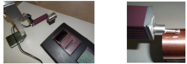
Figure 2: Experimental setup of measuring surface roughness using MITUTOYO SJ-301 surface roughness tester
