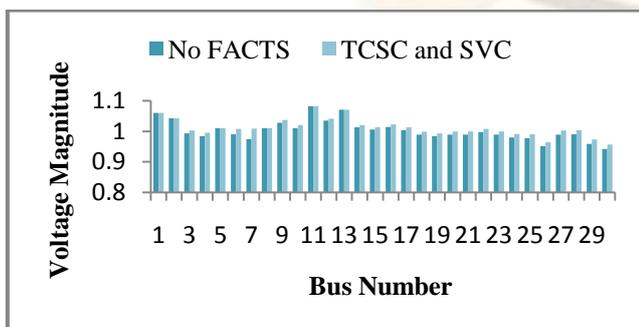
Figure 7: Voltage profile improvement with TCSC and SVC
