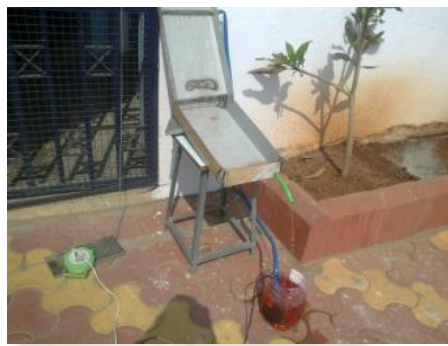
Fig No.2 Experimental set up for photocatalytic treatment
