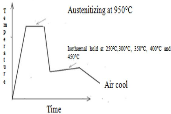
**Fig. 2: Two-step Austempering heat treatment cycle**
