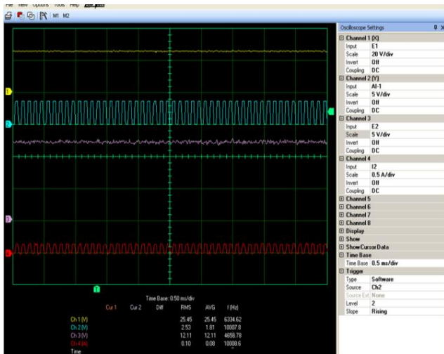
Figure 23. waveforms of output voltage and output current at capacitance value of capacitor 210uF with switching frequency 10,000Hz.
