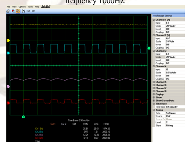
Figure 16. waveforms of output voltage and output current at capacitance value of capacitor 5uF with switching frequency 2000Hz.
