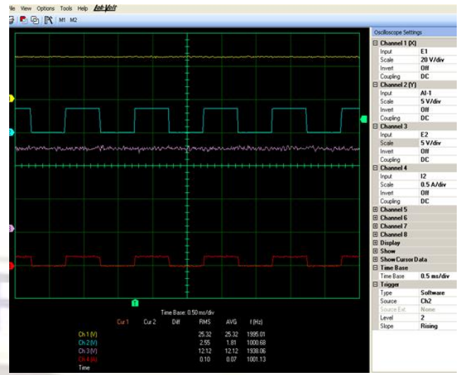
Figure 20. waveforms of output voltage and output current at capacitance value of capacitor 210uF with switching frequency 1000Hz.
