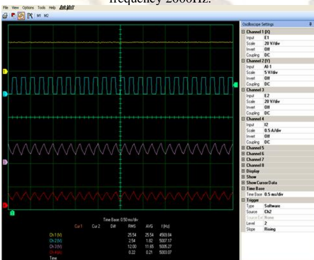
Figure 7. waveforms of output voltage and output current at inductance value of inductor 2mH with switching frequency 5000Hz.
