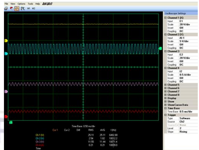
Figure 8. waveforms of output voltage and output current at inductance value of inductor 2mH with switching frequency 10,000Hz.
