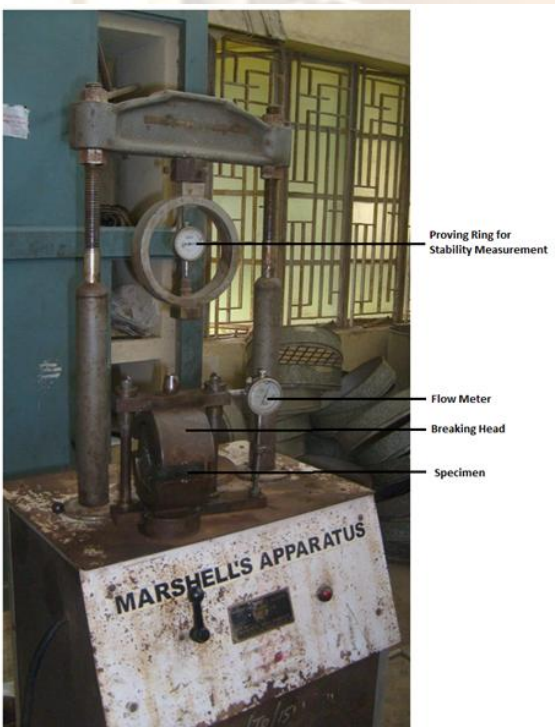
FIG.5 MARSHALL APPARATUS WITH BREAKING HEAD
