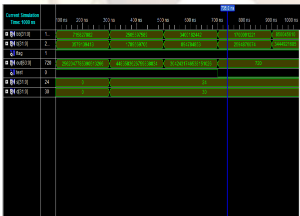
Figure 5:- 32-bit simulation output of BIST TPG for variable precision multiplier
