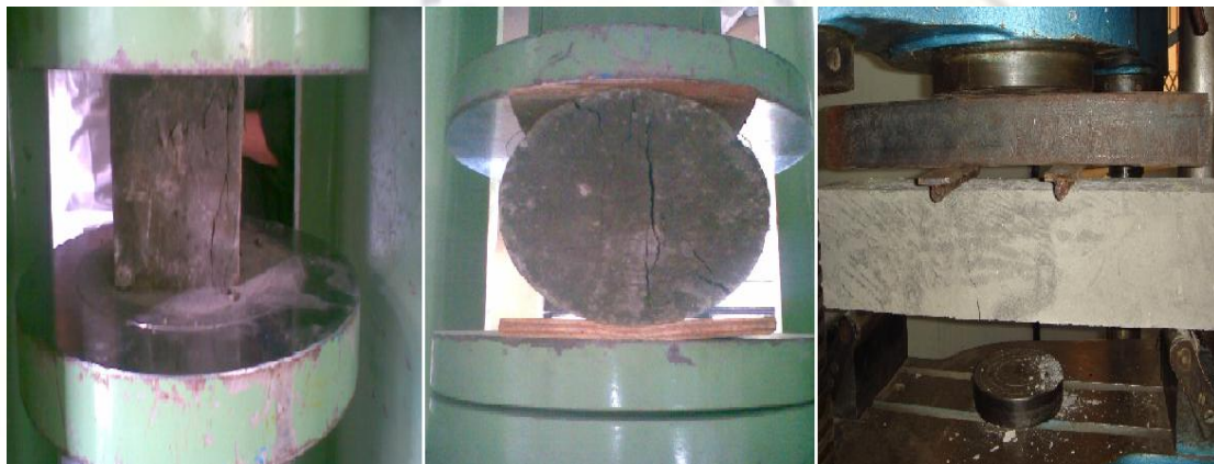
Fig 4. Typical failure patterns
