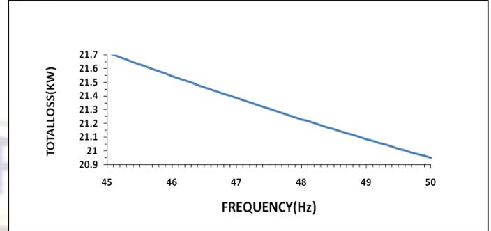
(Fig- 13 Frequency Vs Total loss)
