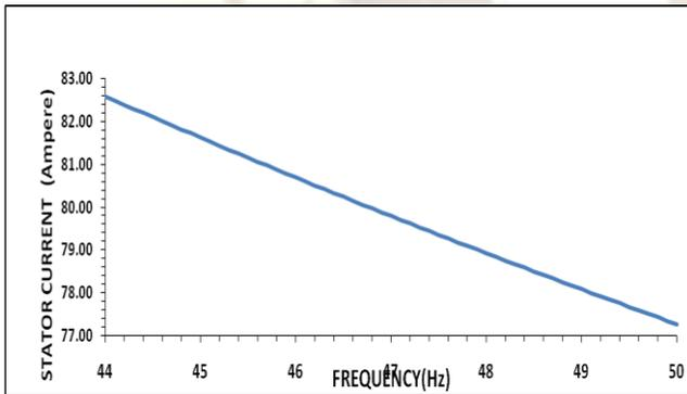
**(Fig-5 Frequency Vs Stator current\_**
