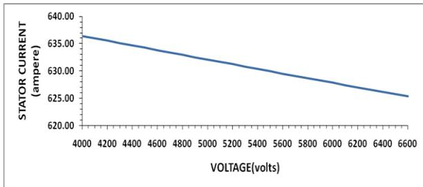
(Fig-9 Stator current Vs Voltage)
