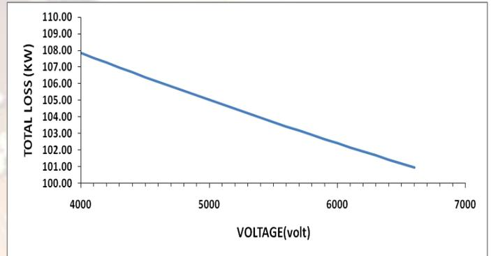
**(Fig- 7 Voltage Vs Total loss)**
