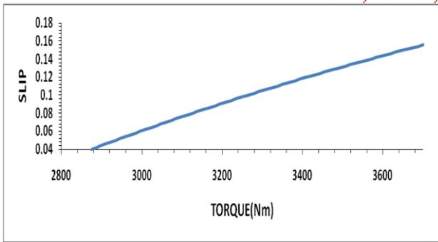
**(Fig- 3 Slip Vs Torque)**
