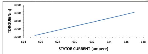
(Fig- 12 Torque Vs Stator current)
