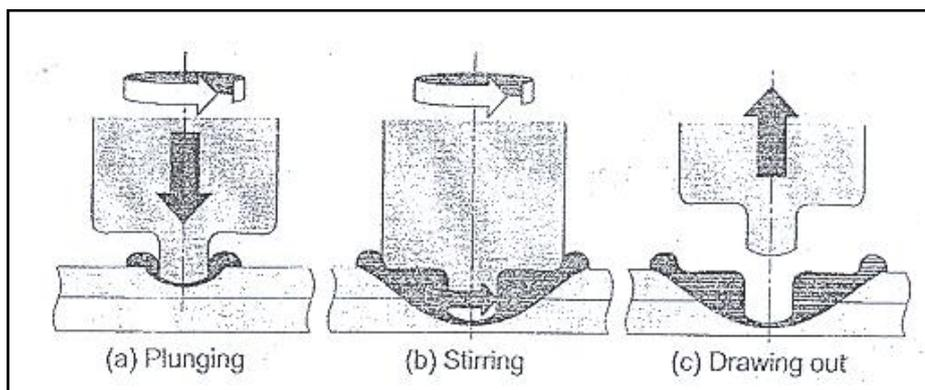
Figure 5 Friction stir spot welding ( FSSW ) steps
