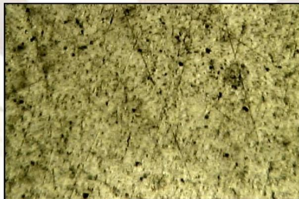
Figure 10 microstructure of base metal after HT and aging at 190°C for 5hr. magnification X125
