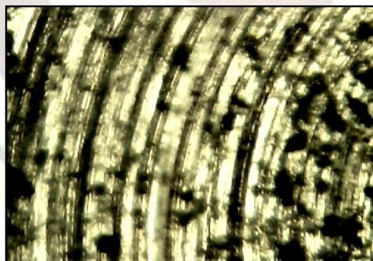
Figure. 7 Onion rings morphology at the tip of the pin of welding tool. Magnification X 63
