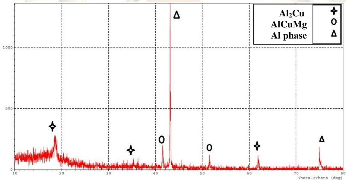
Figure 12 Photograph of XRD analysis pattern of friction stir spot weld after solution heat treatment and aging at 190 °C for 5hrs.
