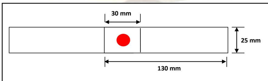
Figure 4 Dimensions of spot weld sample
