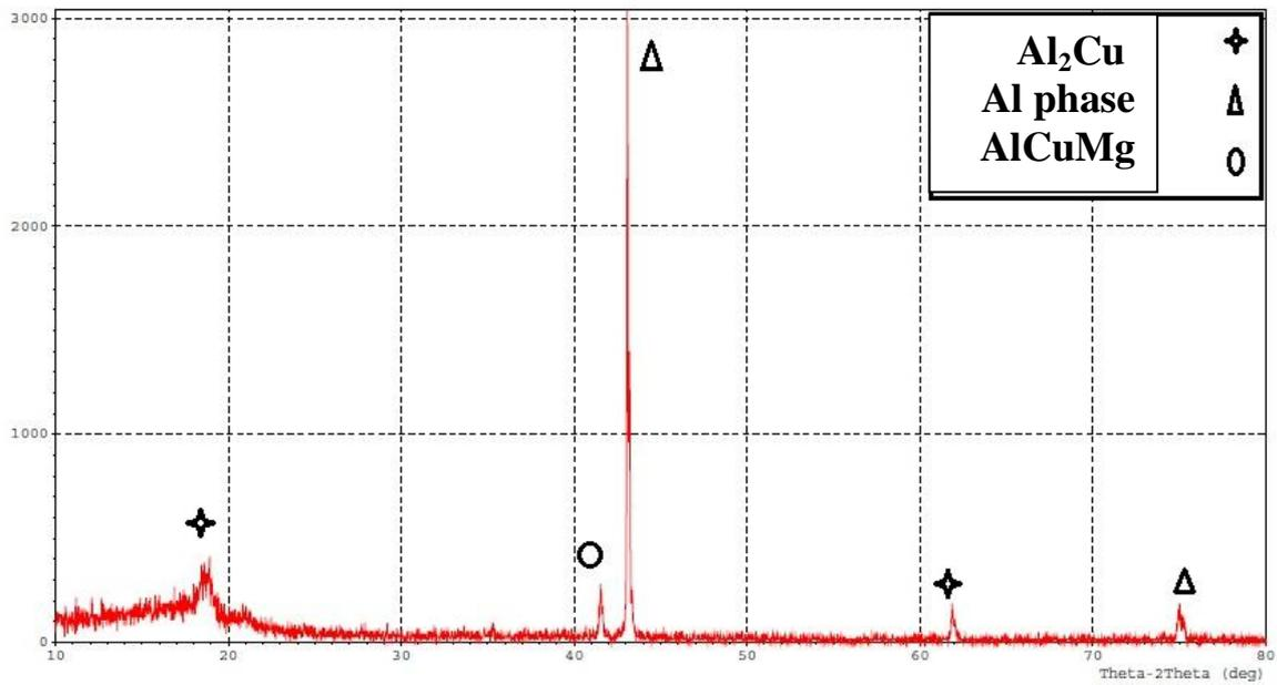
Figure 11 Photograph of XRD analysis pattern of friction stir spot weld before heat treatment ( as weld)
