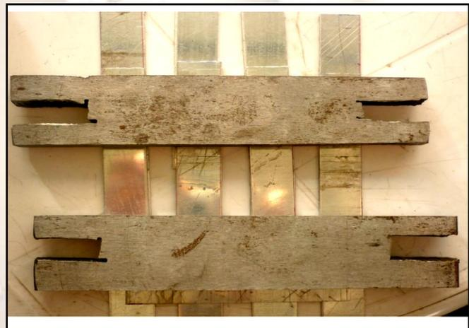
Figure 3 Clamping the Al-alloy plates with fixtures
