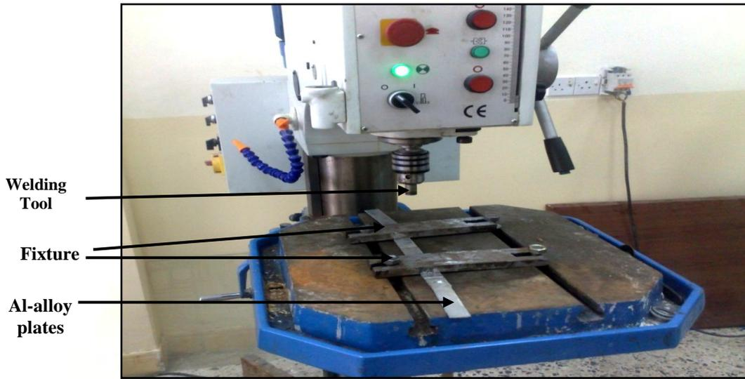
Figure 1 Milling machine used in FSSW in this study
