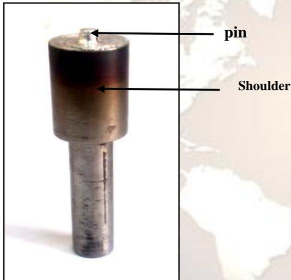
Figure 2 Welding tool (X38) used in this study
