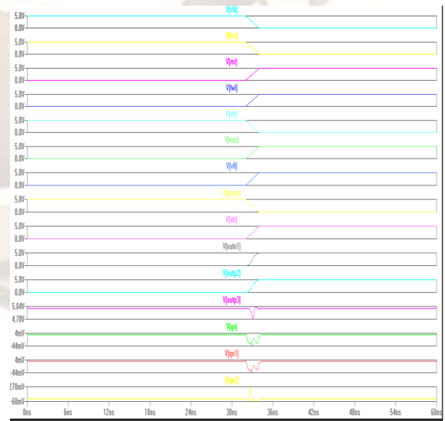
Fig 19 Waveforms of aircraft using dynamic latch comparator (when v_{tr} > (v_{ne}, v_{fl}) )
