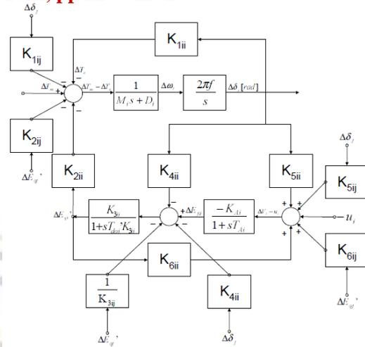
Fig 2 Transfer function block diagram representation of Multimachine system
