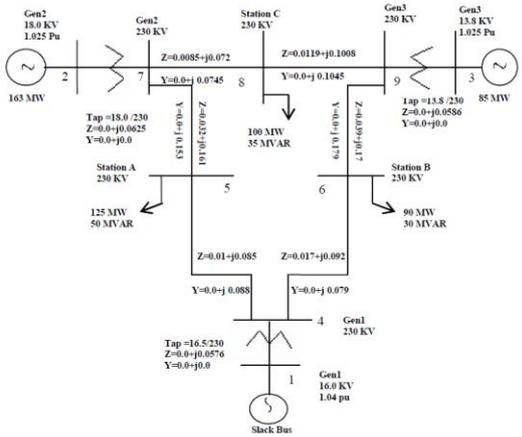
Fig 1: 3-Machine 9-Bus system
