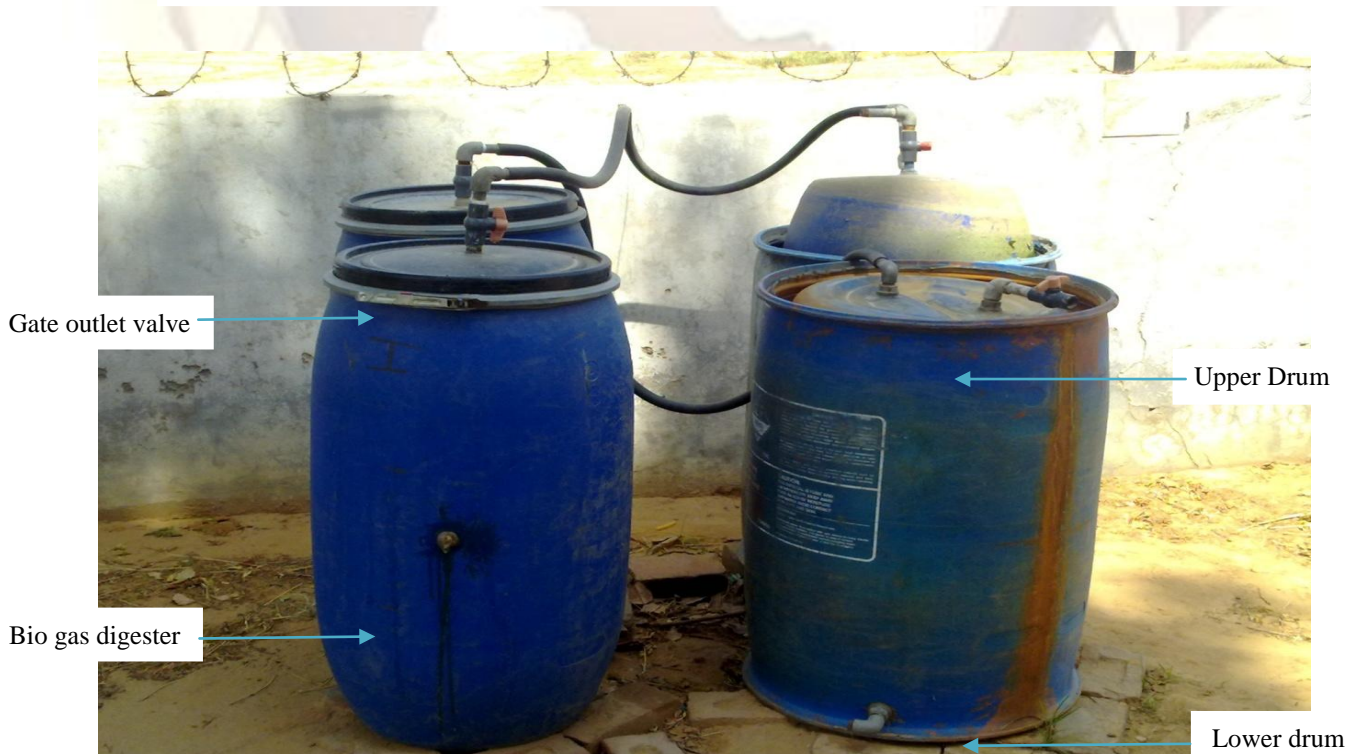
Fig 2: Bio gas digester (Two 124 litre capacity) along with displacement drum
