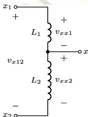
Fig. 2. Tapped Reactor Model
