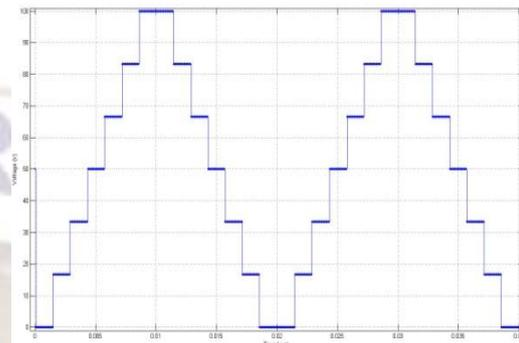
Fig.4 Seven level output
